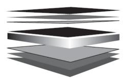
Finish Coat (Nominal 20µm) (Refer Note 4 & 5) Universal Corrosion Inhibitive Primer (Nominal 5µm) Conversion Coating
