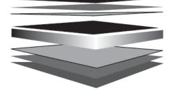
Finish Coat (Nominal 20 $\mu m)$  (Refer Note 4 & 5) Universal Corrosion Inhibitive Primer (Nominal 5 $\mu m)$  Conversion Coating
