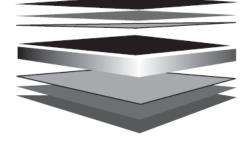
Finish Coat (Nominal 20 $\mu m)$  (Refer Note 4 & 5) Universal Corrosion Inhibitive Primer (Nominal 5 $\mu m)$  Conversion Coating
