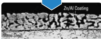
Microscopic view of TRUECORE® steel
