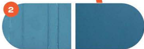
Conventional prepainted steel The steel shows significant colour fading.
