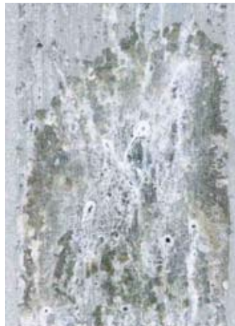
ZINCALUME® steel @ 2000 hours of salt spray testing.
