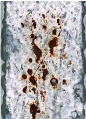
Z275 galvanised steel @ 240 hours of salt spray testing.
