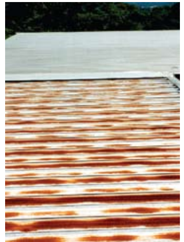
Galvanised steel, foreground, and ZINCALUME® steel after 20 years of natural exposure.
