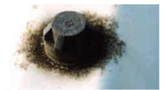
The rubber washer component of screws must be made from materials compatible with the cladding material. Conductive washers are not suitable for use with ZINCALUME<sup>®</sup> steel or Clean COLORBOND<sup>™</sup> steel products. Conductive washers can cause galvanic cell corrosion between the washer and the cladding material.
