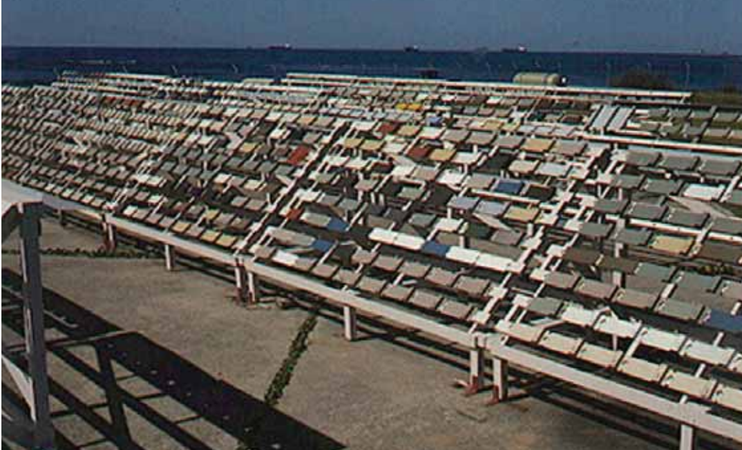
Exterior Exposure- Sample racks at Bellambi Point, NSW, Severe Marine environment.
