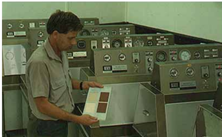
QUV - Used to provide accelerated rates of weathering.
