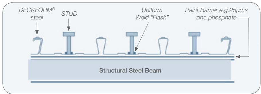
readily welded, and shear studs can be welded through the LGC DECKFORM® steel product in the same manner as regular DECKFORM® steel.
