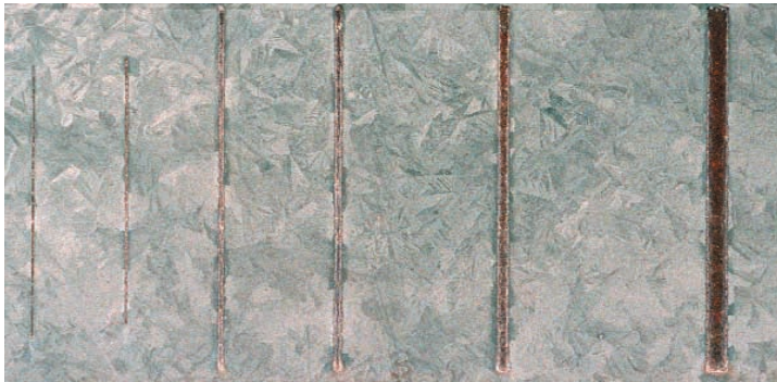
Figure 4: Zinc-coated sample, Z275.
