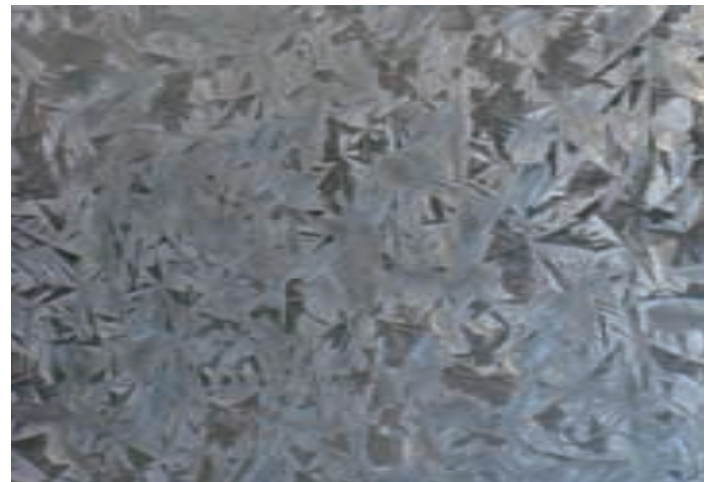
The distinctive "spangle" pattern of galvanised steel
