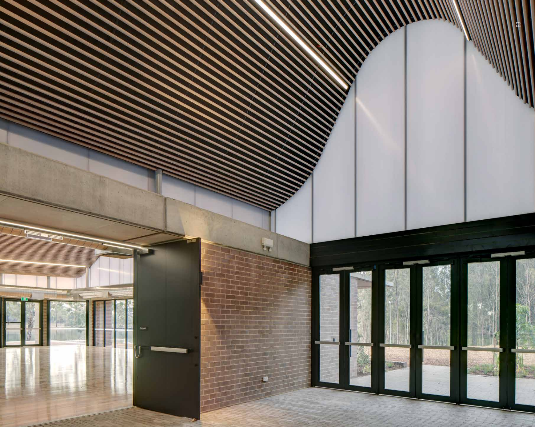
ABOVE: The foyer's southern interior aspect reveals the highest single point of the roof's profile, with the expansive void created by the curve filled with sheets of white opalescent polycarbonate. BELOW: The 3D Model (supplied by A Class Engineering) was instrumental in the success of the entire project, allowing the team to work through the complexities of a profile where curves undulate east to west while the fall runs south to north.
